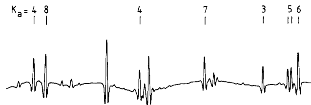
Figure 2. Part of the HCSCN spectrum showing a characteristic pattern with different K_a components of the J:33 \leftarrow 32 transition (together with some lines belonging to an unidentified byproduct); frequency scan 204.2–204.3 GHz.
